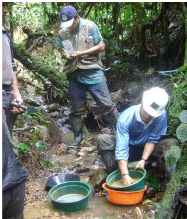
Gambar 4.2. Kegiatan Stream sediment sampling (Sumber; www.doratoresources.com )
