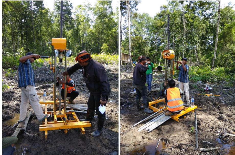
Gambar 5.10 Survei Pengambilan data Sondir
